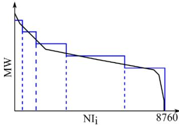
Figure 1. Multi-stage model of the load duration curve
