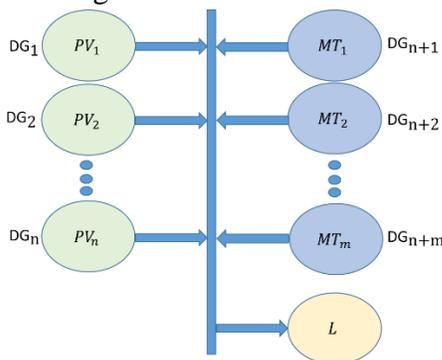
Figure 3. Simple model of the distributed generation system and load ( $DG_1, \dots, DG_{n+m}$  are the nominal generation capacities of  $n$  PV units and  $m$  MT units,  $L$  is the load in a certain time).
