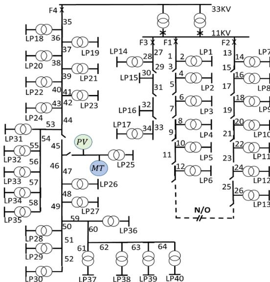
Figure 5. RBTS Bus 6 modified with distributed generation.
